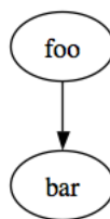
Figure 5.1: Graph of a test suite consisting of two modules, i.e. foo and bar. The arrow represents that bar is imported by foo.
