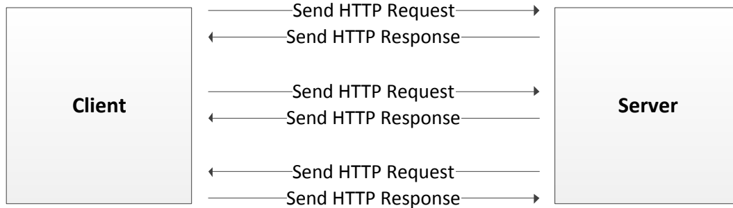
Figure 2.10.: Communication scheme of Web applications.
